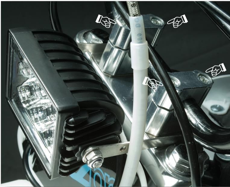
Tighten stem onto the upper crown and route all cables outside the bracket
