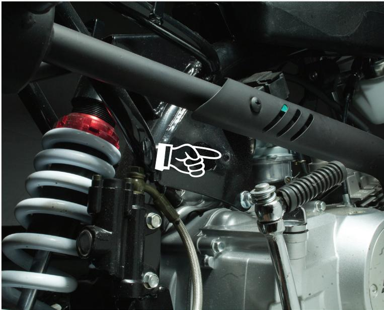
Locate mounting hole on frame behind the exhaust and above the engine.
