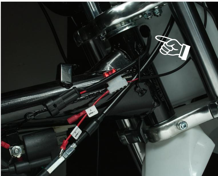
Route light plug through hole in number plate. Plug bullet labeled **B** into male bullet on regulator/rectifier harness
