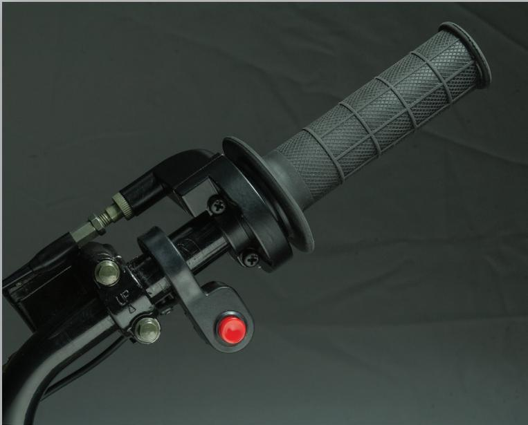
Install switch by removing throttle grip with a Phillips screw driver. Slide switch onto bar and tighten with 2.5mm hex key.
