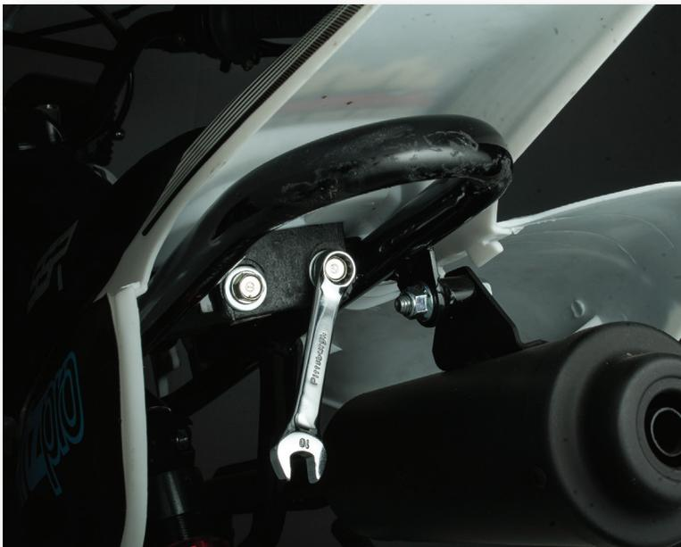
Uninstall the seat by removing the two screws underneath and slide back.
