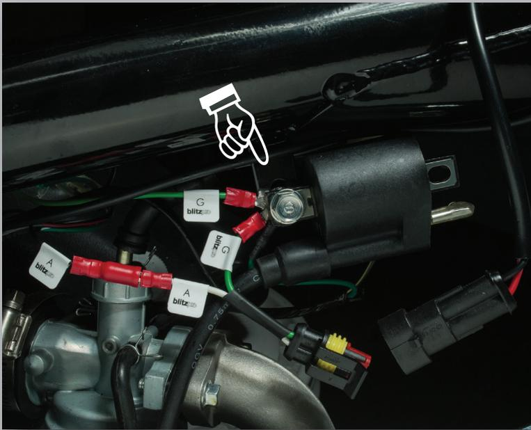
Bolt all green wires labeled **G** to the exposed metal tab located underneath the top tube. Match remaining wires labeled **A** and plug in.
