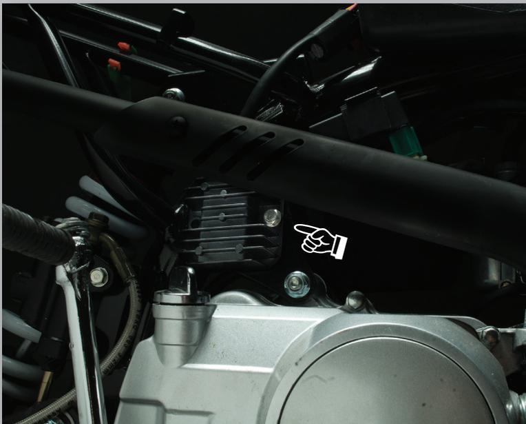
Install regulator/rectifier with the 10mm screw and nut supplied in the kit.
