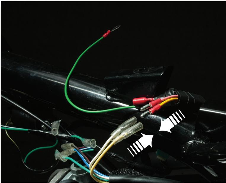
Plug the two male bullet terminals from the regulator/rectifier into the female terminals of the white and yellow wires on the chassis.
