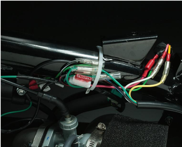
Install new zip tie and re-bundle loose wires to the top tube. Check all wire connections with a light tug.
