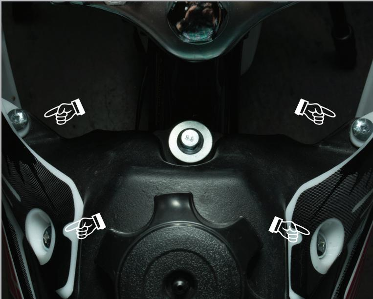
Remove four screws that hold the front of the bike's seat to the fuel tank
