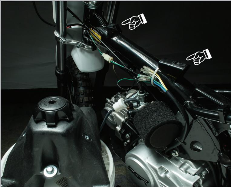
Remove the two screws holding the fuel tank. Cut ziptie to access the wires.
